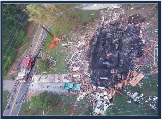
EXPLOSION RESULTING FROM A CROSS BORE IN AUSTELL, GEORGIA
